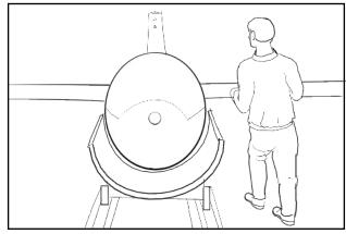
Push the glider out of its support and onto the wheel.
