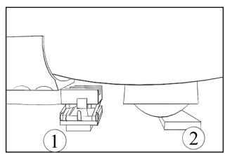
The glider should now roll onto block 2, lifting it over the fuselage support, and setting it down at the right position.
