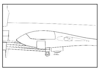
Pull out the fuselage, and extend the undercarage. Block 1 should prevent the wheel from touching the ground, by app. 1 cm Making undercarage extension possible.
