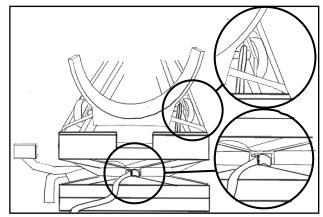
Take the strap and secure the fuselage support. Make sure the pin does not block the support from going into the trailer.
